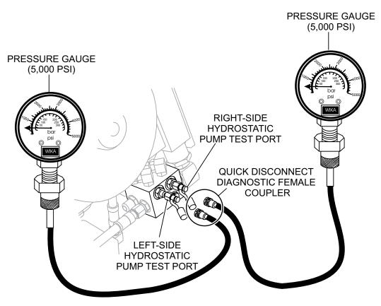
Figure 47. Hydraulic Pump Pressure Test Ports
